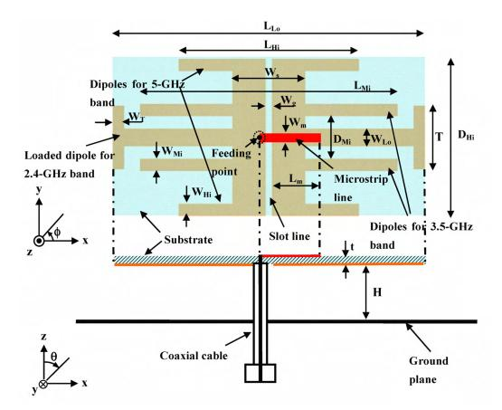
Fig. 1. Configuration of a triple-band unidirectional coplanar antenna.
