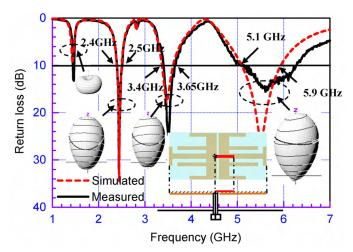
Fig. 2. Simulated and measured results for return loss of the triple-band unidirectional antenna.
