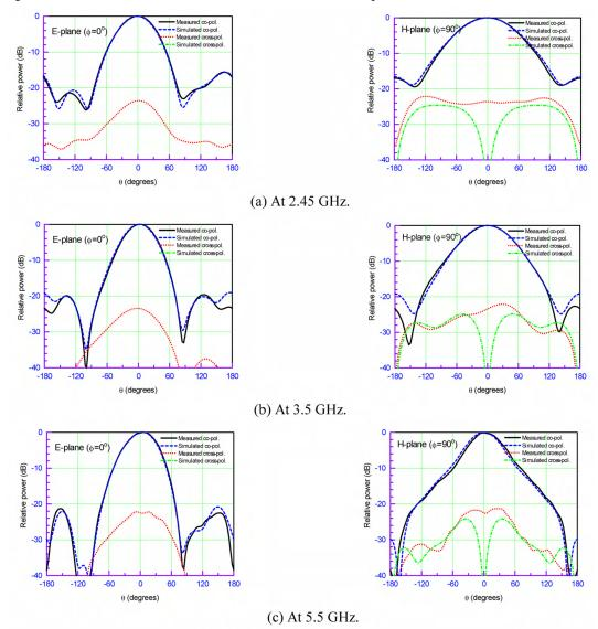
Fig. 3. Radiation patterns of the triple-band unidirectional antenna.
