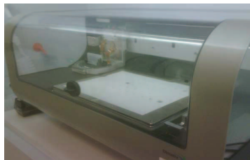
Fig. 4. Dimatix ink-jet printer used to fabricate the antenna.
