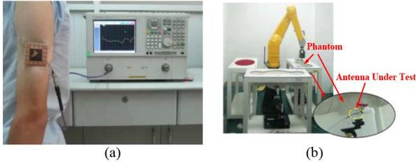
Fig. 6. Photographs of experiments using (a) Agilent N5 230A vector network analyzer and (b) SPEAG DASY5 SAR measurement system.
