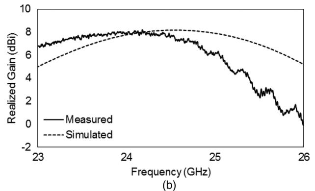
Fig. 5. Simulated and measured realized gain for inkjet-printed (a) 3- and (b) 5-director Yagi-Uda antennas.
