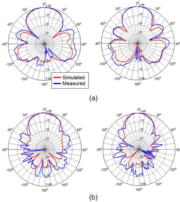
Fig. 6. Simulated and measured normalized (a)  $yz$  and (b)  $xy$  E-field radiation patterns for inkjet-printed (left) 3- and (right) 5-director Yagi-Uda antennas.
