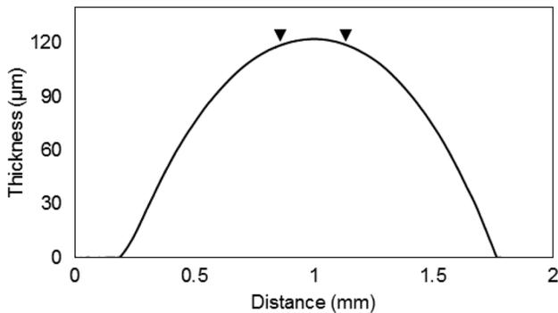
Fig. 3. Profilometer scan of the printed 18-layer ( $120\ \mu\text{m}$  thick) SU-8 dielectric substrate of the microstrip feedline, identifying the  $300\ \mu\text{m}$  area of the printed silver feedline  $\blacktriangledown$ .
