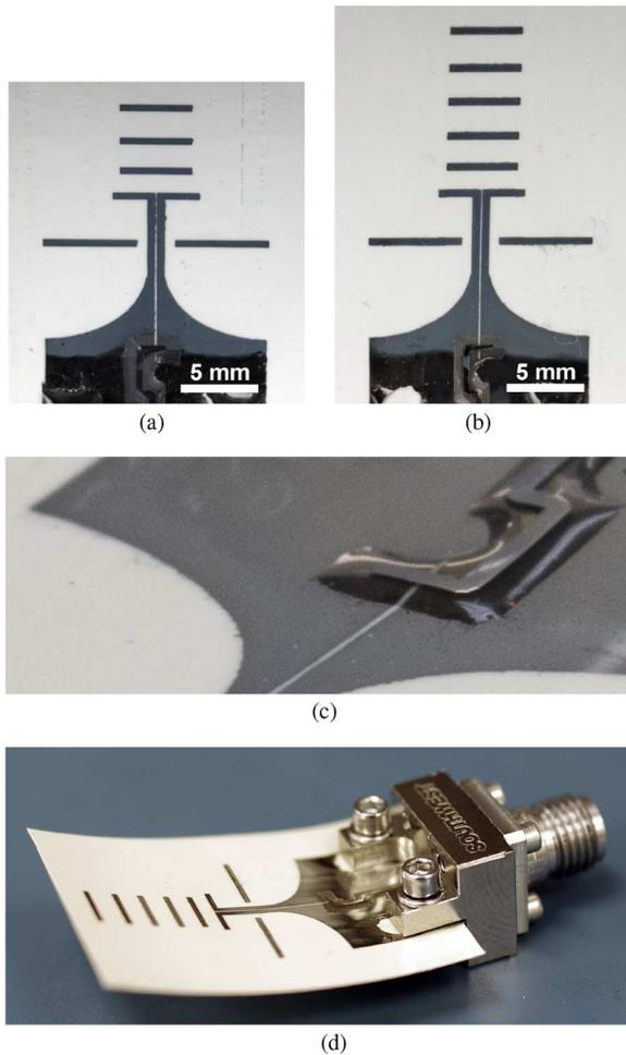
Fig. 2. Inkjet-printed multilayer (a) 3- and (b) 5-director Yagi-Uda antennas with detailed images showing (c) the printed dielectric substrate for the microstrip-to-slotline feeding transition and (d) slight substrate bending.
