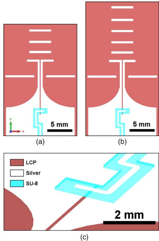
Fig. 1. Simulation models for inkjet-printed (a) 3- and (b) 5-director Yagi–Uda antennas with (c) detail showing a multilayer microstrip-to-slotline transition.
