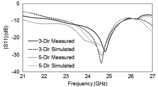
Fig. 4. Simulated and measured return loss values for the inkjet-printed 3- and 5-director Yagi-Uda antennas.
