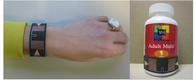
Fig. 2. Picture of fabricated antenna for various conformal applications, like wireless health monitoring and pharmaceutical drug bottle tracking.
