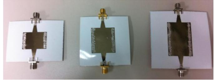
Figure 2. Photograph of the SIW interconnects with different length.
