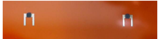
Figure 2. Figure 2. Thin graphene films inkjet-printed in between and overlapping silver conductive inkjet-printed trace on Katpon substrate.
