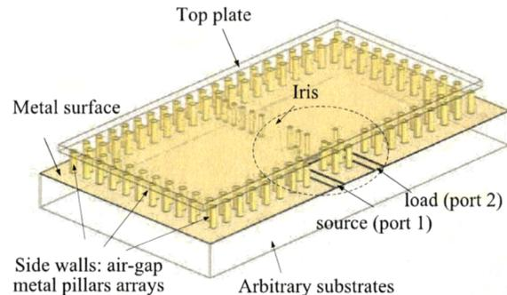
Fig. 1. Concept drawing of the proposed filter structure (detailed structures in the dashed circle is shown in Fig. 2 ).
