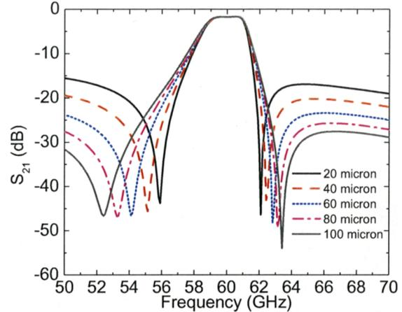
Fig. 4.  $S_{21}$  as the function of the CPW gap in source loading capacitive coupling
