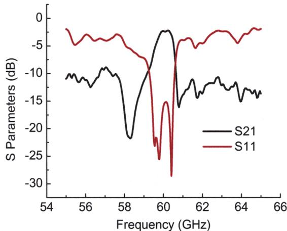
Fig. 8. Measurement results of the fabricated source-load coupling filter
