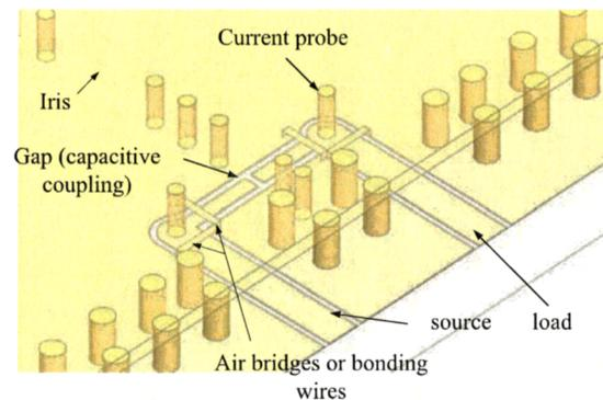
Fig. 2. Feeding and coupling schemes for the proposed filter.
