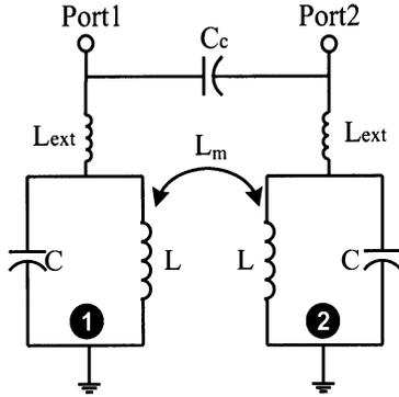
Fig. 3. Equivalent circuit model for the proposed source-loading coupling 2-pole filter
