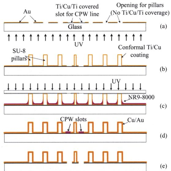
Fig. 6. Fabrication flow of the proposed air-lifted cavity resonator filter.
