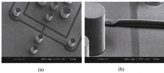
Fig. 7. SEM pictures of (a) feeding and source-load coupling before wire-bonding.(b) a bonding wire span over a CPW slot.
