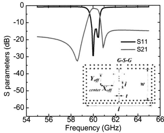
Fig. 5. Optimized filter response and illustration of physical dimensions
