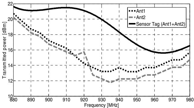
Fig. 5. Sensitivity analysis: minimum required transmitted power for activating individual tag (ant1, ant2) and the sensor (ant1+ant2).
