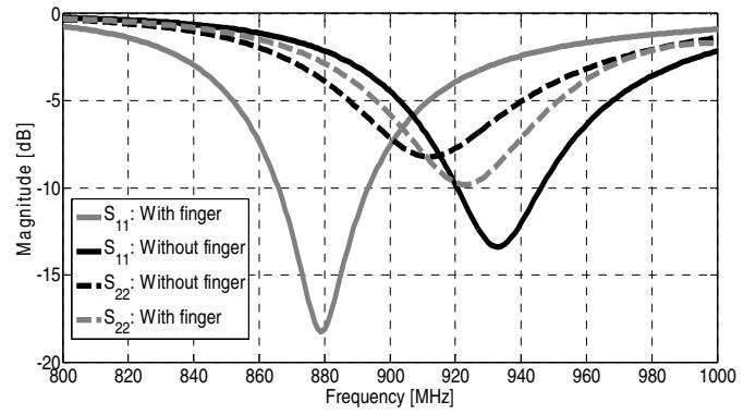
Fig. 3. Simulated input scattering parameters of the two antennas.
