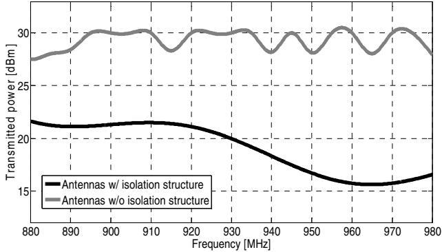
Fig. 4. Measured minimum transmitted power of 2x1 RFID antenna array with/without meta-material inspired isolator.
