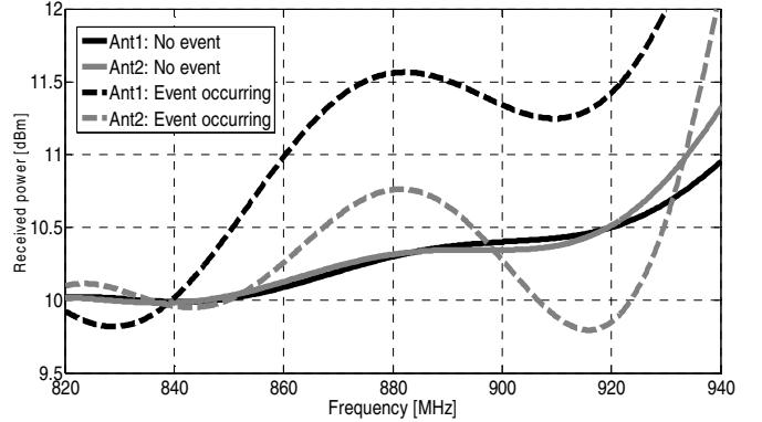
Fig. 6. Measured reflected power from the sensor each element before/after event occurring.
