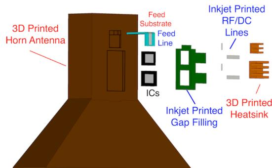
Fig. 1. Exploded view of the of a SoA proof-of-concept topology, demonstrating the many layers needed to be assembled. The ICs are an amplifier and VCO, with the amplifier amplifying the VCO signal to generate a wide range of signals based on the VCO tuning voltage. 3D parts are labeled in red, inkjet parts are in blue.
