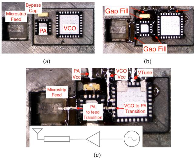
Fig. 2. Fabrication of the chip attachment utilizing inkjet printing. (a) The chips, “L-shaped” microstrip output feed line and bypass capacitor for the PA are placed into the built-in cavity in the antenna. (b) SU8 gap filling. (c) RF and DC inkjet printed lines, with equivalent schematic.
