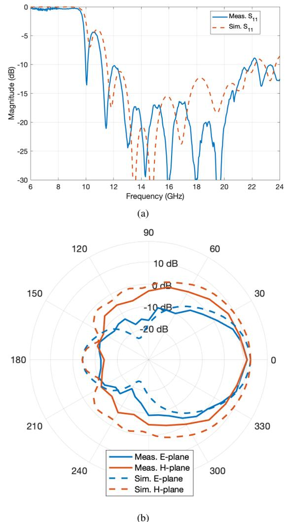
Fig. 4. Simulated and measured horn antenna: (a)  $S_{11}$ , and (b) gain pattern.
