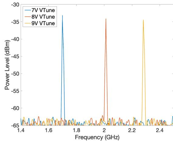
Fig. 6. Received power level from the SoA, with different tuning voltage. The frequency received is 14.7GHz, 15GHz, and 15.26GHz for 7V, 8V and 9V tuning voltage respectively. The frequency measured is post frequency conversion due to the mixer.
