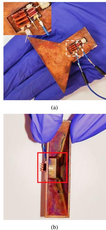
Fig. 3. (a) The top view of the SoA module prototype with enlarged heat sink (inset). (b) Side view clearly showing the L-shaped microstrip feed inside the horn.
