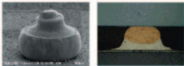
Figure 2 - Picture of flip-chip bump. The flip chip ball before (left) and after (right)
