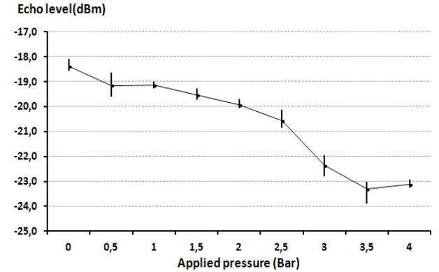
Fig. 4: Measured echo level of passive EM pressure sensor versus applied pressure at the beat frequency  $f_{ant}$  of the antenna scattering mode.
