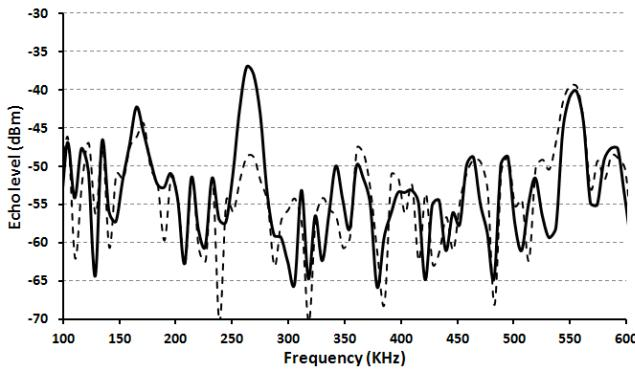
Fig. 6: Measured beat frequency spectrum in the out-door environment shown in Fig. 5 for two extreme values of the physical quantity  $\varphi$ : for  $\varphi = \varphi_1$  (---) and for  $\varphi = \varphi_2$  (—).
