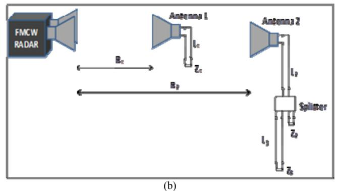
Fig. 7: (a) Proof-of-concept set-up for demonstrating the feasibility of the wireless identification of passive sensors based on the same millimetre-wave FMCW-RADAR used for remote sensing and (b) Schematic of the experimental set-up (the load impedance  $Z_1$ ,  $Z_2$  and  $Z_3$  are infinite).
