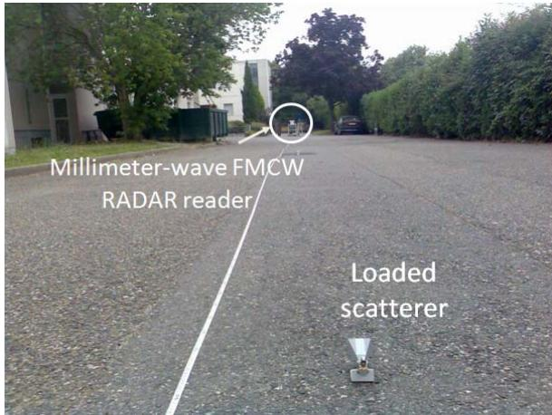
Fig. 5: Outdoor environment for the measurement of the beat frequency spectrum synthesized by a FMCW RADAR operating at 29,75 GHz. The scatterer is placed on the ground surface at 30m from the RADAR.
