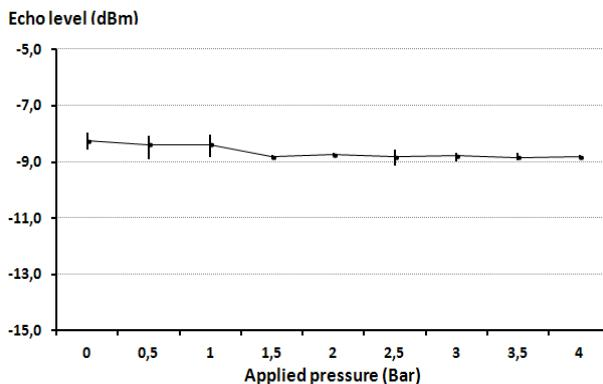
Fig. 3: Measured echo level of passive EM pressure sensor versus applied pressure at the beat frequency  $f_{str}$  of the structural scattering mode.
