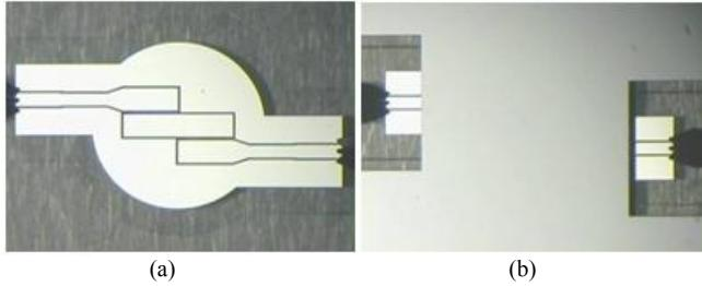
Fig. 1: Top views of the first passive pressure-sensing device based on electromagnetic transduction and operating in the millimetre-wave frequency range (dimensions:  $3.8\text{mm} \times 5.8\text{mm} \times 1.4\text{mm}$ ): (a) the planar half-wavelength resonator deposited inside a circular Pyrex cavity and (b) the high resistivity silicon membrane placed at the top of the planar resonator.
