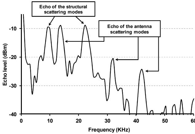
Fig. 8: Beat frequency spectrum synthesized by the millimetre-wave FMCW RADAR Reader when interrogating the scatterer shown in Fig. 7.
