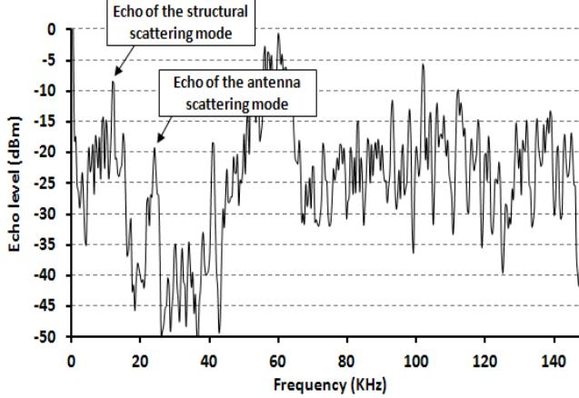
Fig. 2: Measured beat frequency spectrum synthesized by the RADAR reader when the pressure is not applied on the sensing device.
