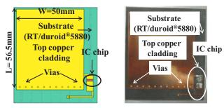
Fig. 4. The (a) designed and (b) fabricated RFID-enabled prototype smart skin strain sensors.
