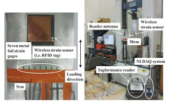
Fig. 5. (a) Sensor instrumentation, (b) Tensile tests setup
