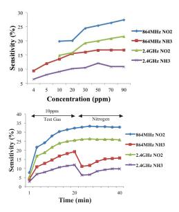
Fig. 8. (a) Response as a function of concentration taken after stabilization and (b) Timing response for NH<sub>3</sub> and NO<sub>2</sub> using concentration of 10 ppm at 864 MHz and 2.4 GHz.
