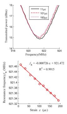
Fig. 6. Tensile testing results for the  $\sim 20~\mu \epsilon/\text{step}$  loading case at an interrogation distance of 12 in. (a) Average transmitted power threshold, (b) Resonance frequency  $f_R$  versus strain  $\epsilon$ .
