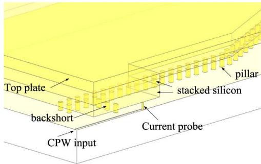
Fig. 2. The close-up schematic for the feeding structure (split along the symmetry plane).
