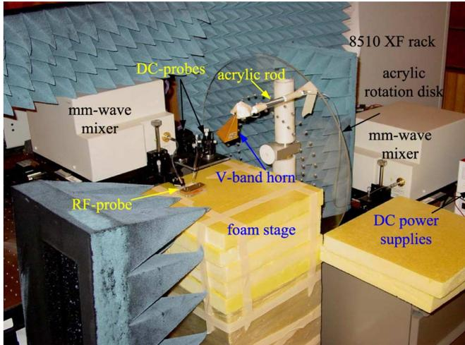
Fig. 11. On-wafer pattern measurement setup.
