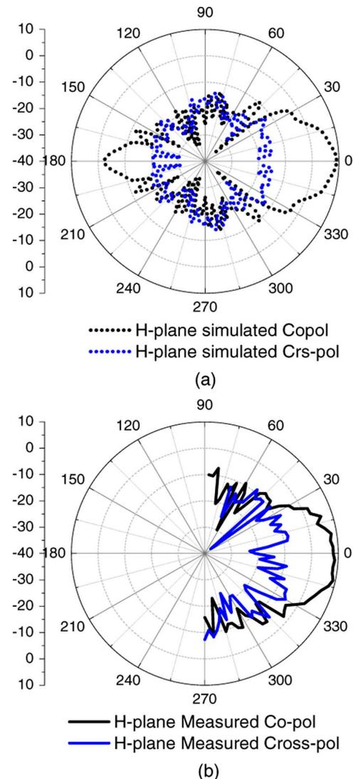
Fig. 13. (a) Simulated and (b) measured H-plane gain patterns.
