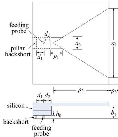
Fig. 3. Illustration of horn dimensions (top and side views).
