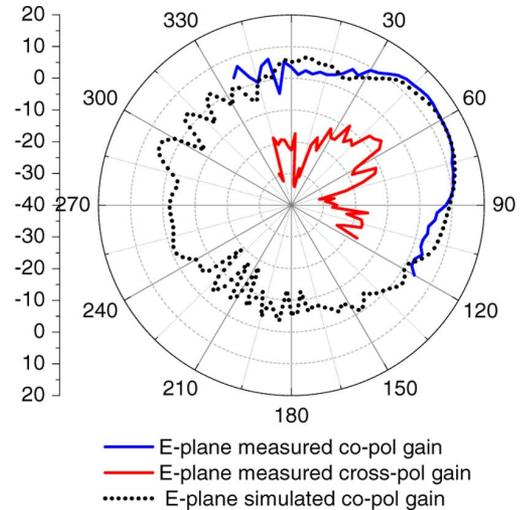
Fig. 12. Simulated and measured E-plane gain patterns.
