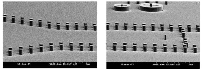
Fig. 8. SEM pictures for the micromachined horn showing the feeding probe and the horn flare pillar sidewall.
