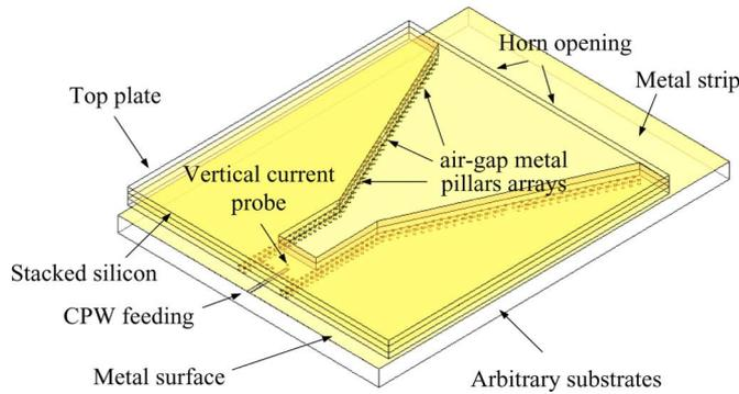
Fig. 1. 3-D view of the proposed micromachined horn.
