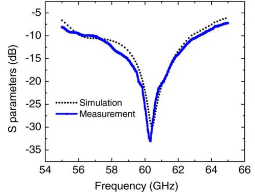
Fig. 5. Simulated and measured return loss of the proposed horn.
