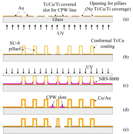
Fig. 7. Fabrication flow of polymer-core-conductor pillars.
