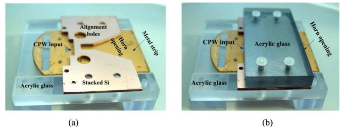
Fig. 10. Pictures of the horn antenna assembly.
