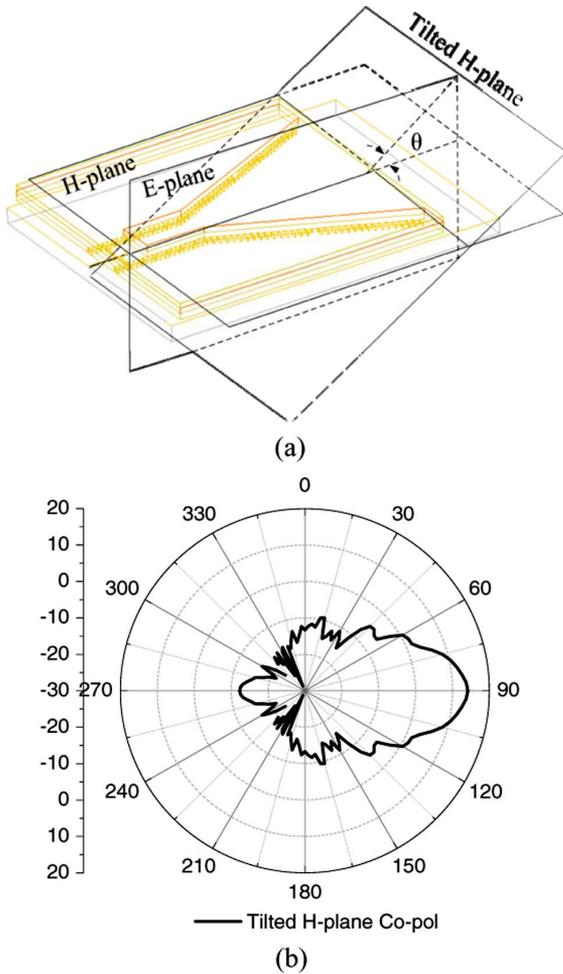
Fig. 6. Radiation pattern cut planes definition and simulated radiation pattern on tilted H-plane.
