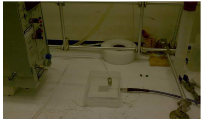
Fig. 16. Closed test cell connected to gas generator and PNA.
