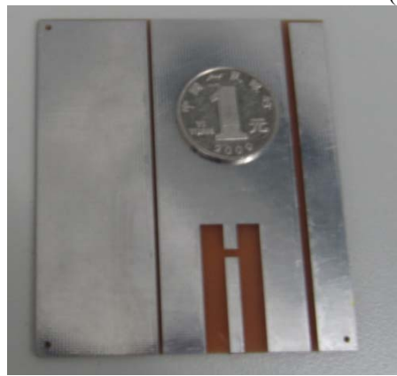
Fig. 1. Configuration of the proposed broadband antenna: (a) Antenna A with one parasitic patch, (b) Antenna B with two parasitic patches, (c) A photograph of Antenna B.
