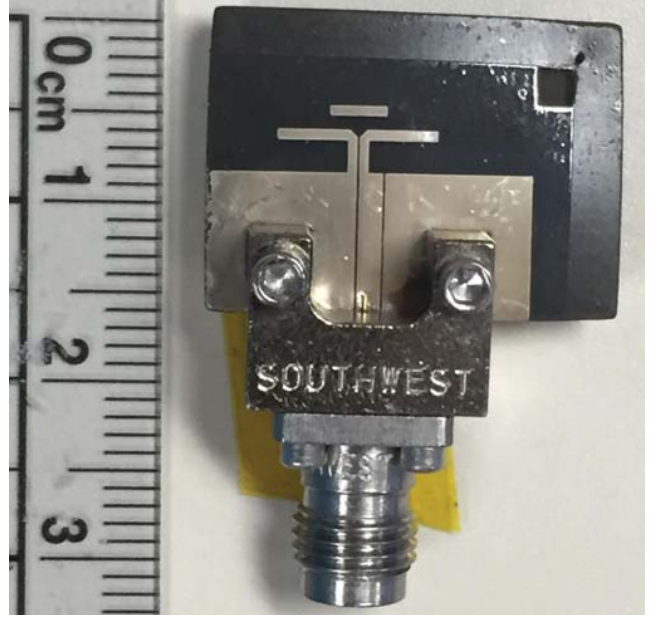
Figure 11. Inkjet and 3D printed broadband on-package antenna.
