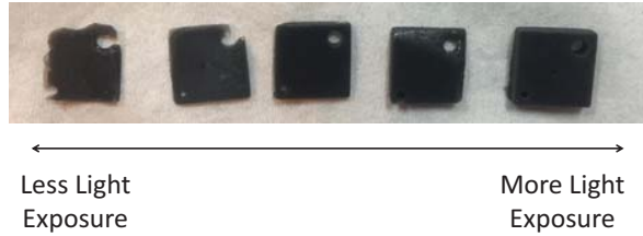
Figure 2. The effects of exposure time on the 3D printed substrates.
