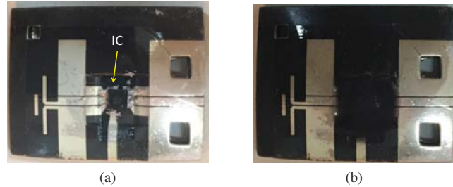
Figure 18. SoP design (a) with IC attached and (b) seal with flexible material
