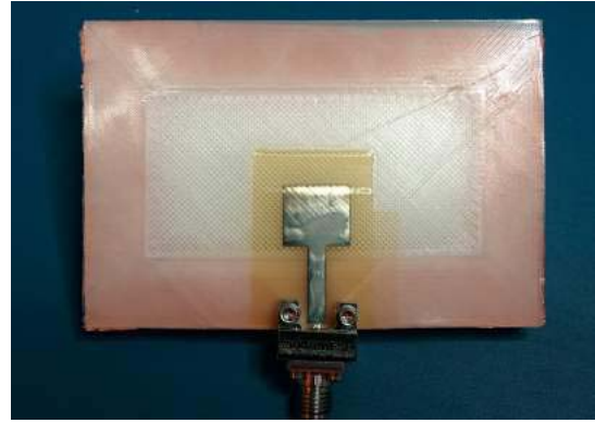
Fig. 6. Photo of the additively manufactured cavity-backed UWB slot antenna.
