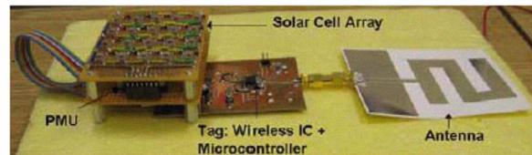
Fig 6. Working tag prototype.
