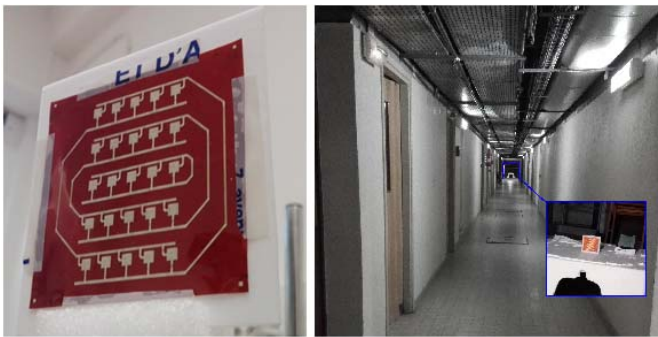
Fig. 1. (a) Kapton-based Van-Atta reflectarray prototype and (b) long range (60 meters) and indoor remote measurement setup of this structure in a corridor.
