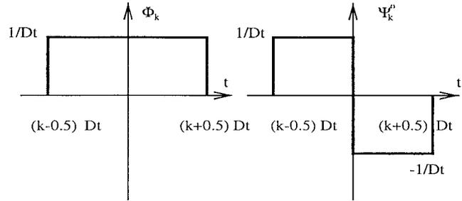
Fig. 1. Zero-order intervalic function basis.
