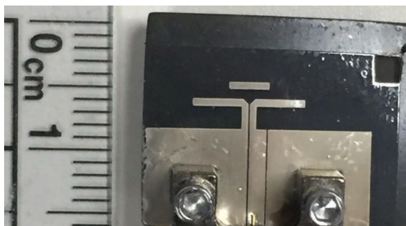
Figure 9. An inkjet- and 3D-printed broadband AiP design [14].
