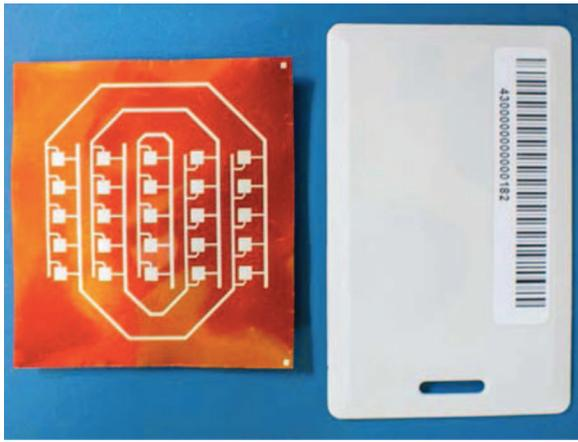
**Figure 7.** An inkjet-printed 30-GHz Van-Atta array prototype compared to a traditional credit card-sized RFID tag [22].
