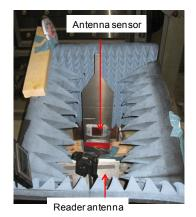
(a) Front view (test specimen is enclosed by foams) (b) Top view Fig. 6. Experimental setup for temperature chamber test
