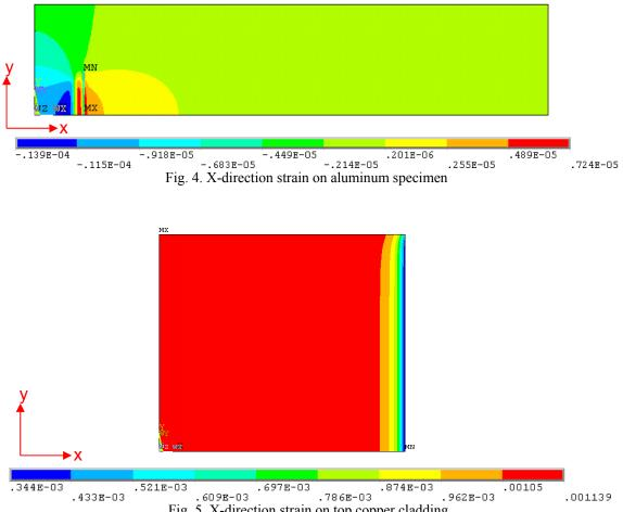
Fig. 5. X-direction strain on top copper cladding
