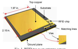
Fig. 1. RFID tag as an antenna sensor
