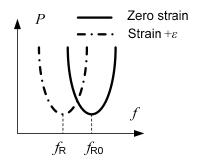
Fig. 2. Conceptual illustration of interrogation power threshold measurement
