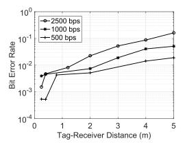
Fig. 17. Measured BER versus the tag-RX distance for 0.5, 1, and 2.5 kb/s.
