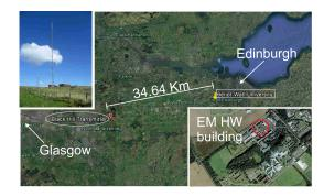
Fig. 12. Scotland FM radio outdoor deployment. The BBC 95.8-MHz station in "Radio 2" band was selected for measurements. The FM transmitter was 34.5 km away from the measurement's setup and its transmission power was 250 kW.
