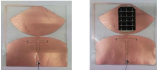
Fig. 1 Photo of the implemented rectennas (a) dual band rectenna 850 MHz / 1850 MHz. (b) dual band solar rectenna 850 MHz / 1850 MHz.
