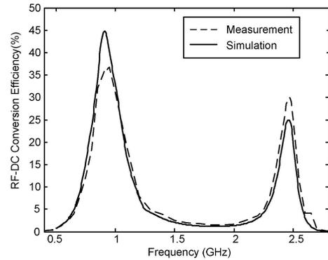
Fig. 4 RF to DC conversion efficiency of the dual band rectenna at 915 MHz/2.45 GHz.
