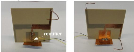
Fig. 3 Photo of the implemented dual band rectenna 915 MHz / 2.45 GHz
