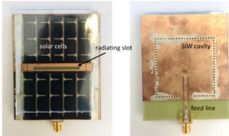
Fig. 6 Photo of the solar SIW slot antenna.
