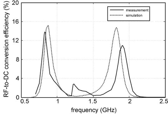
Fig.2 RF to DC conversion efficiency of the dual band rectenna 850 MHz / 1850 MHz.
