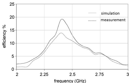
Fig. 7 Simulated and measured RF to DC conversion efficiency of the 2.45 GHz solar rectenna.
