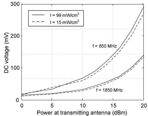
Fig. 5 DC voltage of the solar rectenna for different light intensities.
