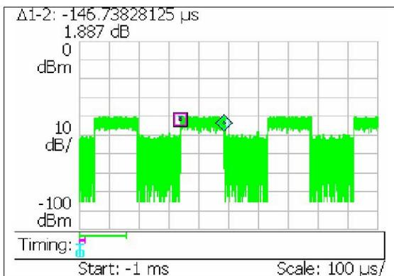
Figure 5. RTSA Measured ASK modulated signal with 50% duty cycle. (Power vs. Time)
