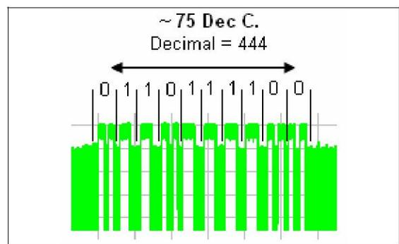
Figure 8. RTSA Measured signal modulation for sensor output at 75° Celsius. (Power vs. Time)
