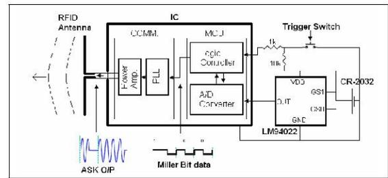
Figure 3. Circuit Schematic of RFID module.
