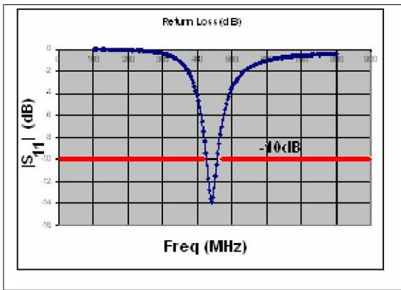
Figure 2. Return loss (dB) of inkjet printed U-shaped antenna on paper.
