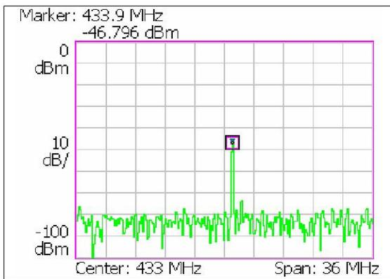
Figure 4. RTSA Received ASK modulated signal with 50% duty cycle. (Power vs. freq.)
