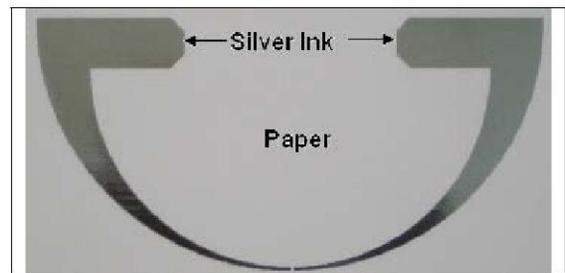
Figure 1. Silver based half-wavelength tapered-width U-shaped antenna
