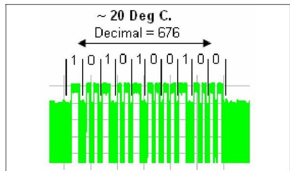
Figure 7. RTSA Measured signal modulation for sensor output at 20° Celsius. (Power vs. Time)
