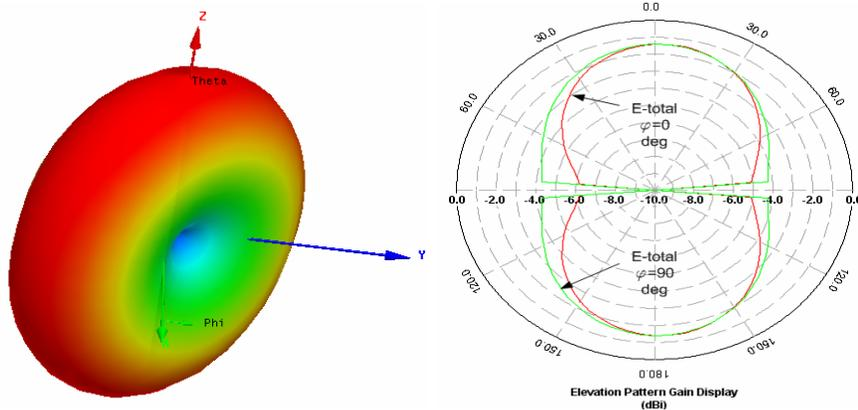
Figure 4. 3-D and 2-D far-field radiation plots.
