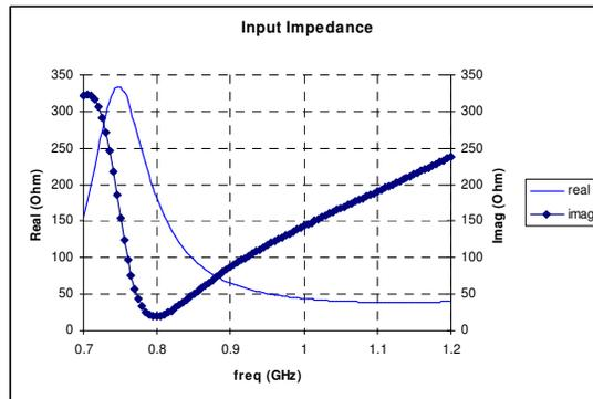
Figure 3. Input impedance of the simulated RFID antenna
