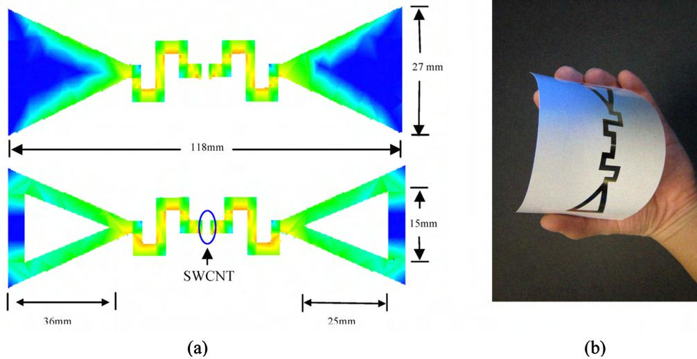
Fig. 2. The RFID tag module design on flexible substrate: (a) current density distribution of the proposed antenna configurations (b) photograph of the fabricated conformal tag.
