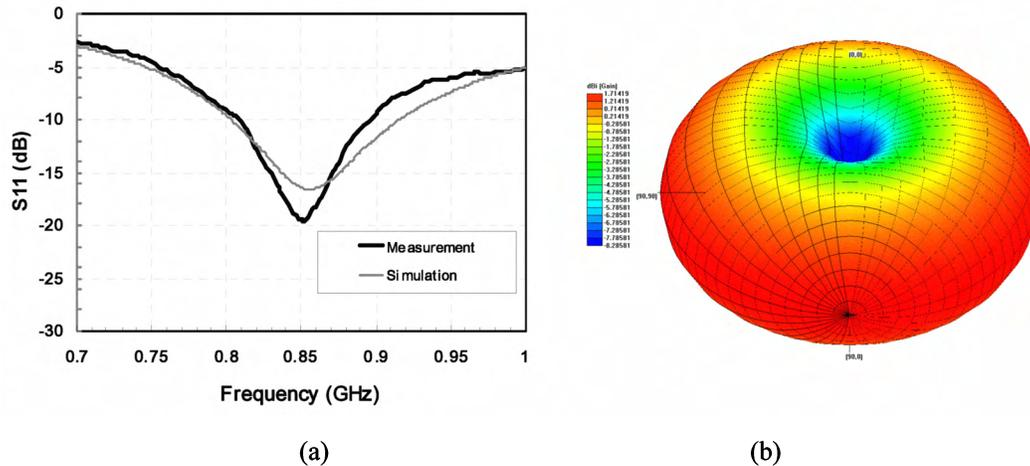
Fig. 3. (a) Measured return loss of the SWCNT-enabled RFID tag antenna (b) Simulated far-field radiation pattern plot. An omnidirectional radiation pattern can be observed at  $\Phi = 0^\circ$  plane with directivity 2.01dBi.
