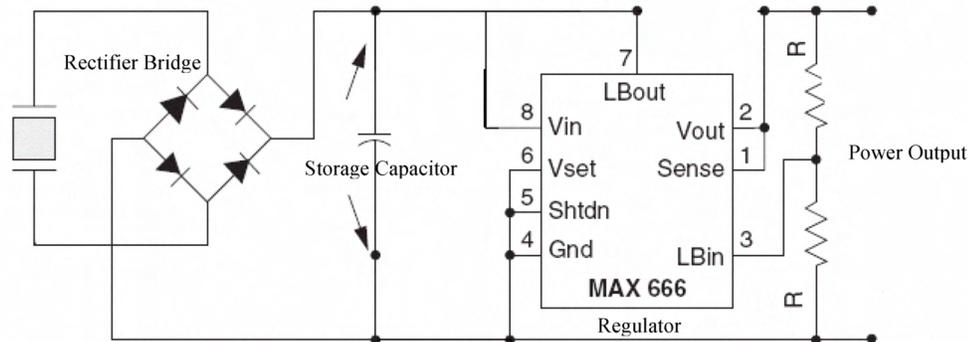
Fig. 4. Piezoelectric scavenger schematic.
