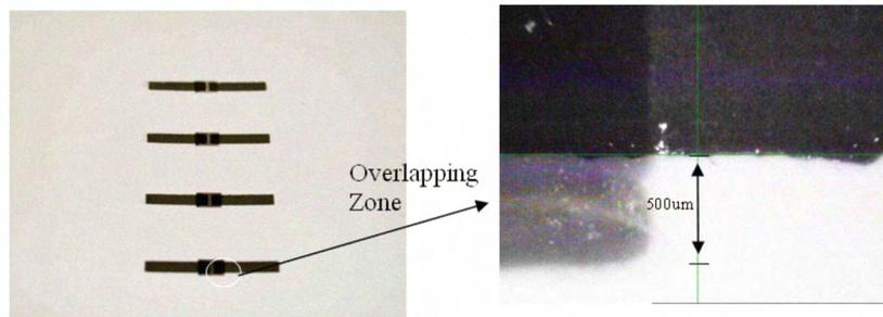
Fig. 1. Photograph of the inkjet-printed SWCNT films with silver electrodes.
