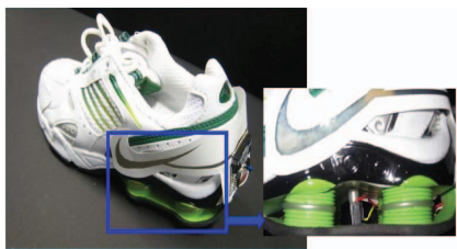
Fig. 6. Self-powered RFID shoes with mounted electronics.
