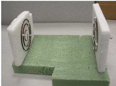
Fig. 3. Measurement setup of the Multiband SCMR system.
