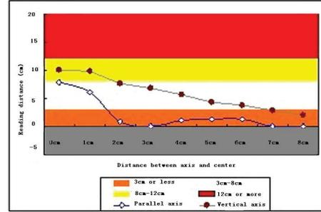
Fig. 6. Reading distances of the tag antenna in 8 positions: perpendicular to the central axis of the turnstile and parallel to the central axis of the turnstile.
