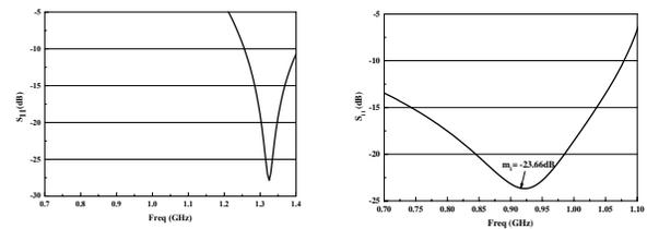
Fig. 2. Reflection coefficient diagram: the left is simple tag antenna model, the right is proposed tag antenna.
