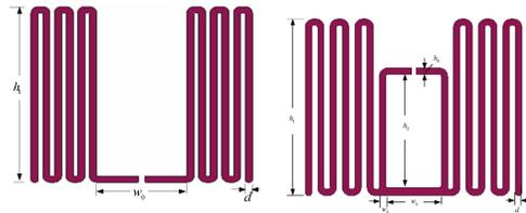
Fig. 1. Antenna model: the left is simple tag antenna model, the right is proposed tag antenna model
