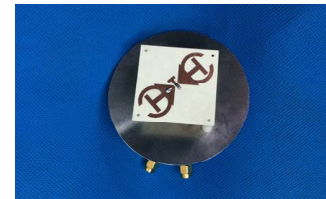
Fig. 2. A prototype of the dual-polarized antenna.
