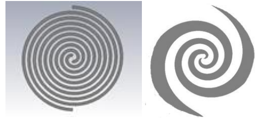
Figure 1. ARCHEMEDIAN SPIRAL (LEFT) AND AN EQUIANGULAR SPIRAL (RIGHT).
