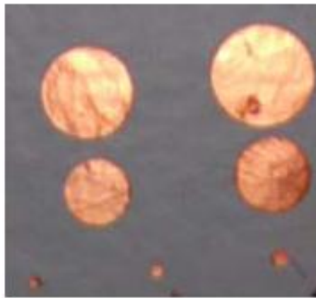
Figure 6. Parallel plate capacitors on 1 mm thick paper substrate.
