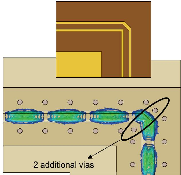
Fig 2. Schematic of CPWG bend.
