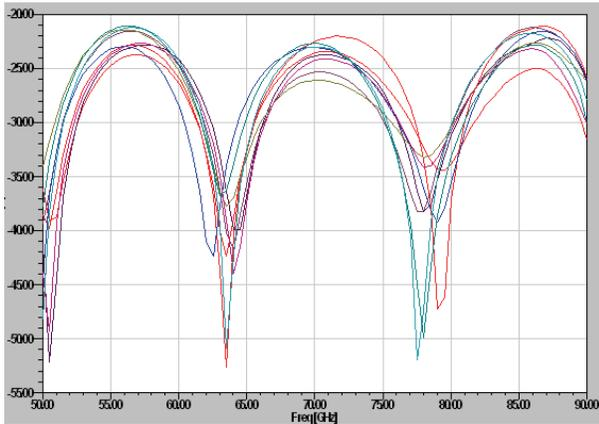
Fig 5. Simulated Return Loss (dB) vs. Freq (GHz) of various positions of vias (sensitivity analysis).
