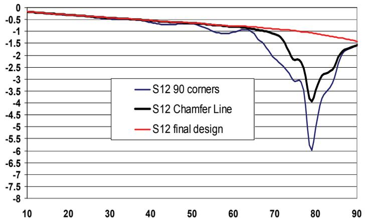
Fig 4. Simulated Insertion Loss (dB) vs. Freq (GHz) of various 90° CPW bends.
