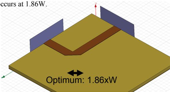
Fig 6. Schematic of optimum 90° microstrip bend.
