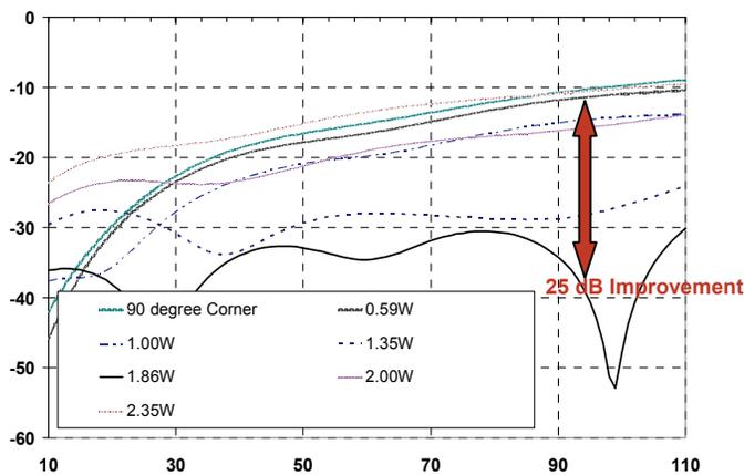
Fig 7. Simulated Return Loss Response of several cases of bending microstrip line.
