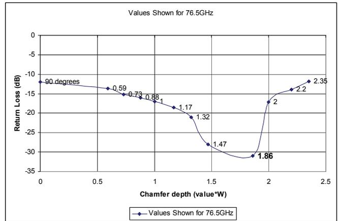
Fig 8. Variation of Return Loss vs. chamfer depth.
