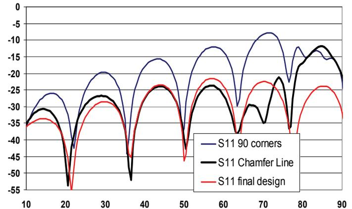
Fig 3. Simulated Return Loss (dB) vs. Freq (GHz) of various 90° CPW bends.
