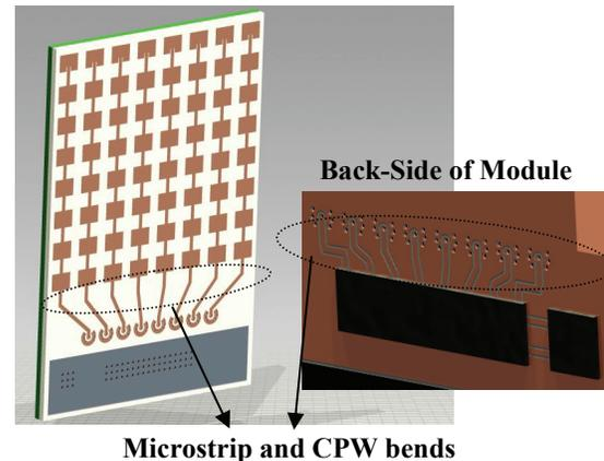
Fig. 1. Schematic of the proposed 3D radar RF front-end showing the location of the microstrip and CPW bends.
