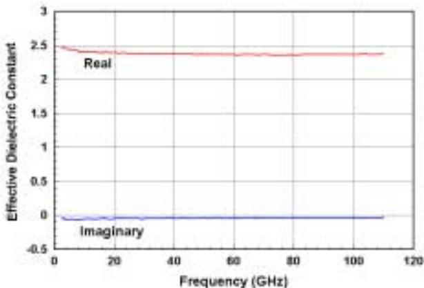
**Figure 4.** Real and imaginary effective dielectric constant versus frequency
