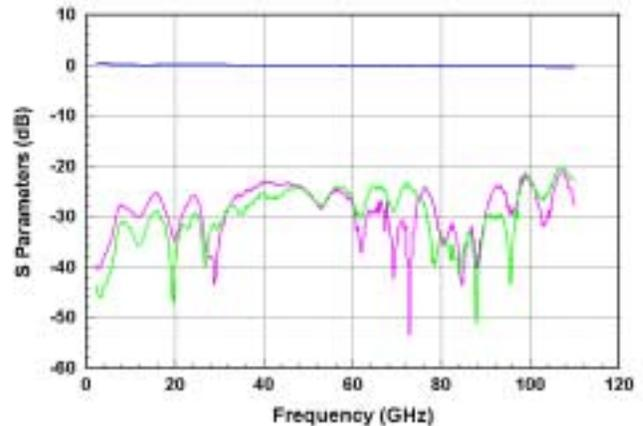
**Figure 6.** S-Parameter Measurement Data of the 0.24 cm line after calibration
