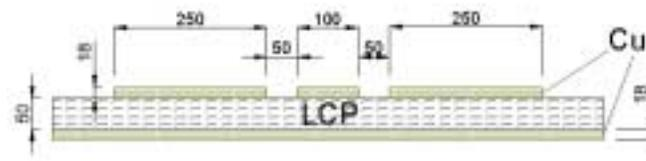
**Figure 1.** CBCPW designed for optimal W-band TRL measurement.
