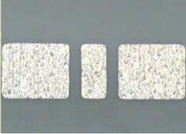
**Figure 2.** Photo of CBCPW transmission line on LCP.
