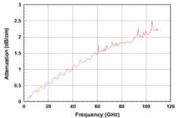
**Figure 3.** Attenuation vs. Frequency for 50  $\mu\text{m}$  LCP substrate CBCPW
