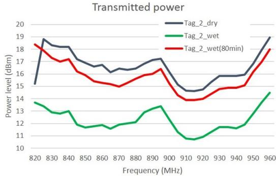
Fig. 6. Minimum transmitted power to activate the prototype tag for different wetting conditions.
