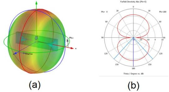
Fig. 4. Simulated radiation pattern of the proposed tag antenna (a) 3D view (b) XZ plane view.
