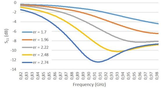
Fig. 3. Simulated reflection coefficient of the proposed tag antenna.
