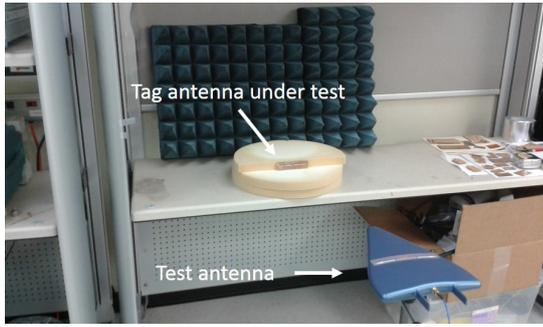
Fig. 5. Measurement setup of the UHF RFID tag antennas tested.
