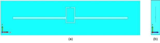
Fig. 1. Simulation model of the proposed RFID tag antenna (a) front view, (b) side view.
