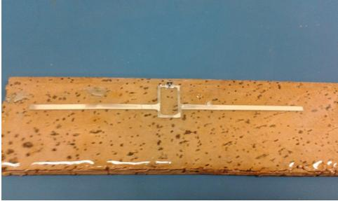
Fig. 2. Prototype photograph of the proposed RFID tag antenna.
