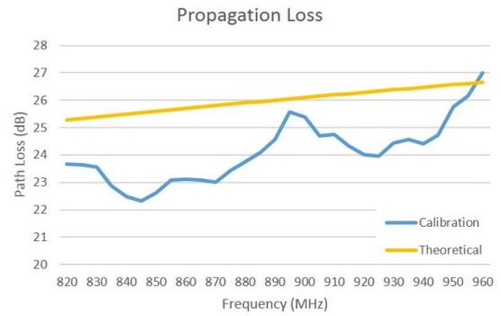
Fig. 8. Theoretical prediction and measured propagation channel comparison.
