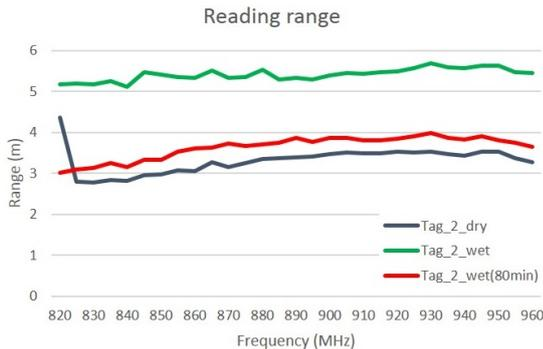
Fig. 7. Reading range obtained for the proposed prototype considering the calibration channel.
