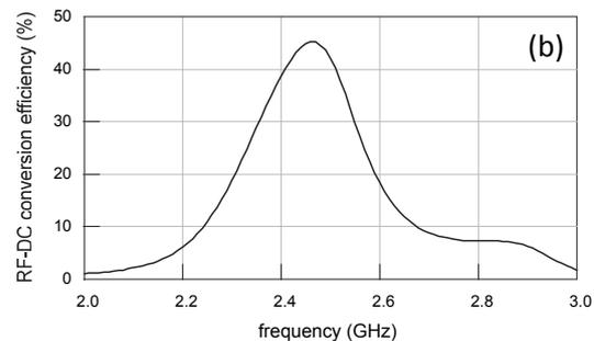
Fig. 7. Rectenna performance (a) S-parameters, (b) RF-DC conversion efficiency.
