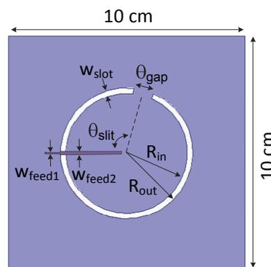
Fig. 1. Shorted ring slot CP antenna (original design).
