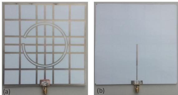
Fig. 5. Antenna prototype, a) top side (meshed ground plane and slot), b) bottom side (microstrip feed line).
