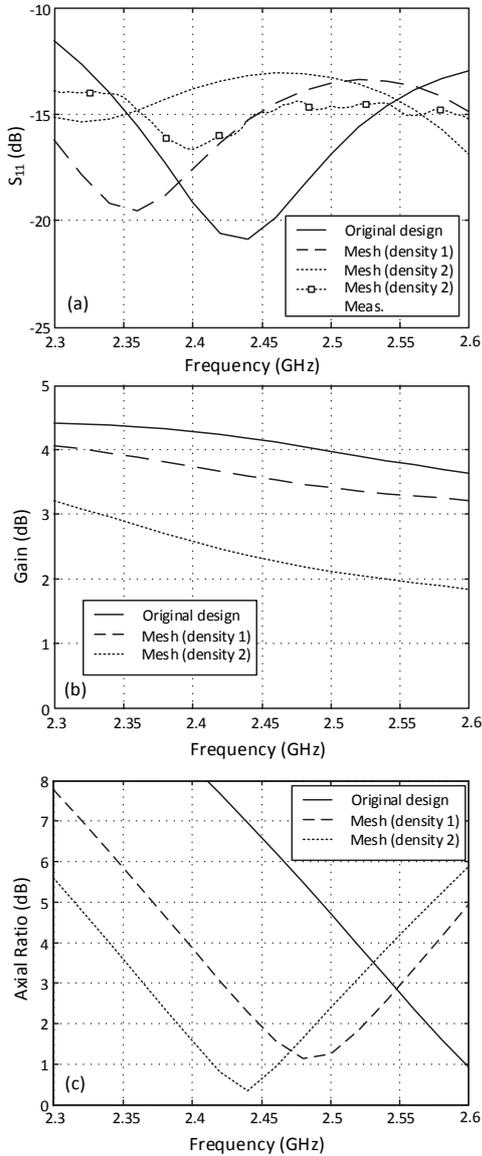
Fig. 2. Performance of the circularly polarized shorted ring slot antenna. (a) Input S-parameters (b) Gain (c) Axial Ratio.
