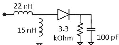
Fig. 6. Rectifier circuit schematic.
