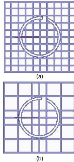
Fig. 3. Shorted ring slot circularly polarized antenna. (a) mesh design with density 1 (b) mesh design with density 2 .
