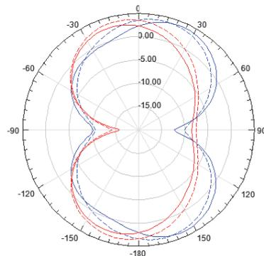
Fig. 4. Simulated gain radiation patterns of the antenna: zy-plane (red), zy-plane (blue), mesh (density 1) dashed line, mesh (density 2) solid line. The antenna feed is along the y-axis.
