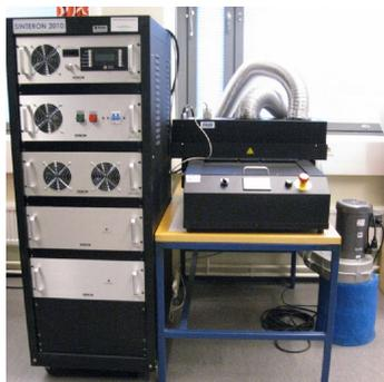
Fig. 1. Xenon Sinteron 2010-L photonic sintering system.
