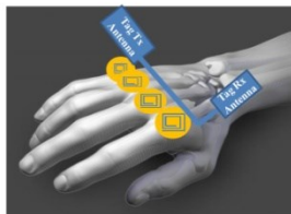
(a) The coding of each hand gesture for 4-resonator circuit (b) Layout of 4 resonators with Tag Tx/Rx antennas Fig. 2. RFID hand-gesture sensor tag
