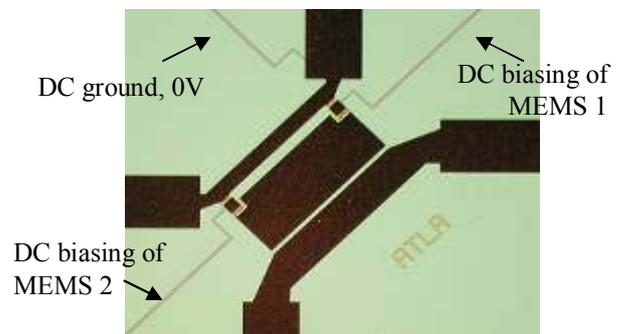
Fig. 5. Picture of the device, with zoom on the coupler. The size of the coupler is 1.4X1.2mm, without feeding lines
