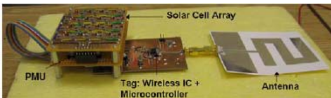
Fig. 7 Working prototype of Solar Powered Battery-less Tag
