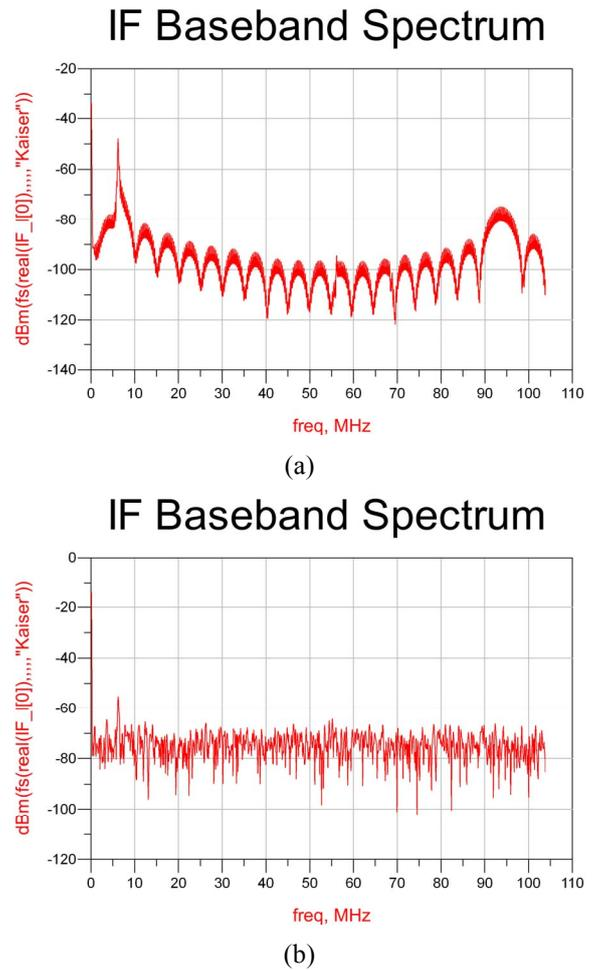
Fig. 7. ADS beat frequency spectrum (a) ideal (b) with noise and coupling.
