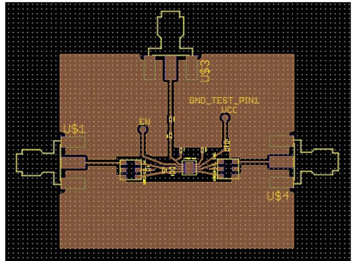
Fig. 3. Inkjet Footprint for Mixer Circuit
