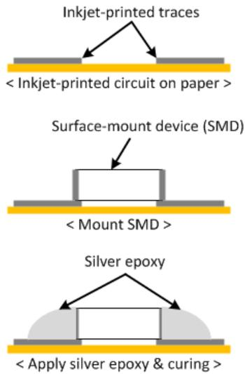
Fig. 5. Mounting process of SMD components
