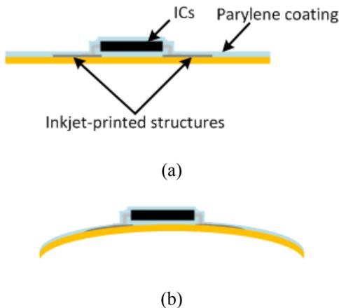
Fig. 6. Parylene coated circuit (a) before bending (b) after bending.
