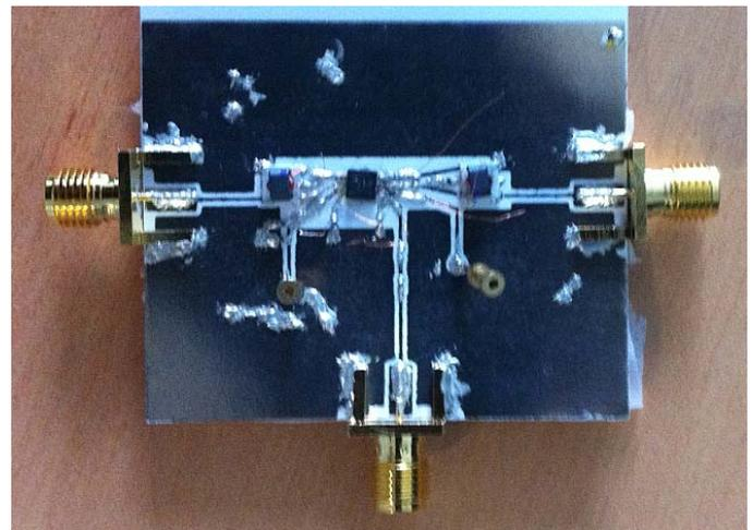
Fig. 4. Paper-based Mixer Circuit
