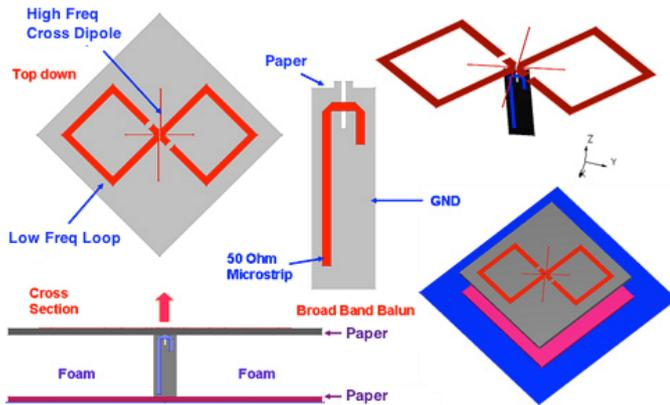
Fig. 8. Dual frequency CP rhombic Loop with crossed dipole.
