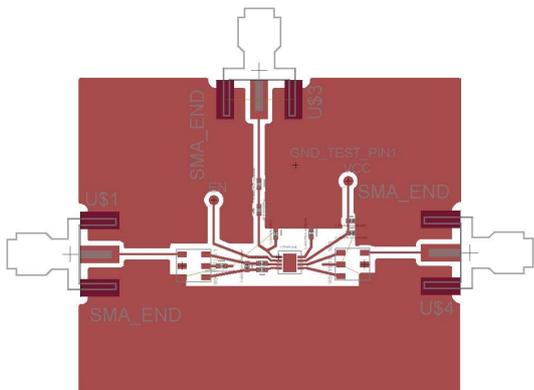
Fig. 2. Mixer Circuit layout in CadSoft Eagle.
