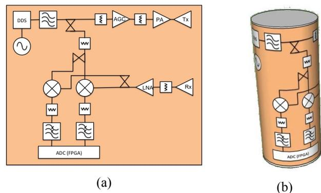
Fig. 1. System level *schematic* illustration of portable radar concept
