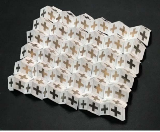
Fig. 4. Fabricated prototype of the 6x6 eggbox metamaterial array.
