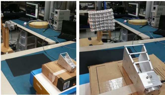
Fig. 5. Measurement setup for for the characterization of the eggbox FSS prototype.
