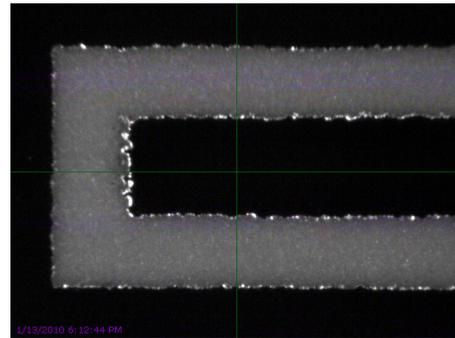
Fig 2. Realized feature size of 50 microns.
