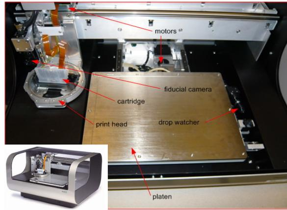
Fig 1. Details of Material Printer DMP 2800 [3].
