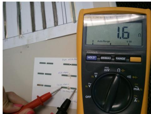
Fig 3. DC characterization for inkjet printed traces with epoxy and SMD 1 $\Omega$  Resistor.
