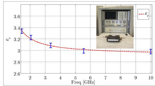
Fig 4. Characterization of the paper material through the split ring resonator method.
