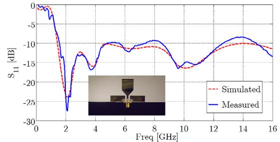
Fig. 5 Simulated and Measured S11 performance of the UWB Antenna.
