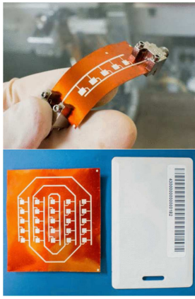
Fig. 2. Additively manufactured inkjet-printed, Smart-Skin humidity sensor tag fabricated with inkjet printed technologies on flexible 7 mils LCP ( = 3.14, \tan = 0.0025 ). The presented system combines the low-cost AMT, mmID, and Frequency Modulated Continuous Wave (FMCW) enabling next-generation ultra-low power, wearable, wireless posture and gesture recognition systems. Thus, through the use of AMT, wearable, flexible realizations of mm-Wave devices provide tremendous potential in future biomonioring applications.
