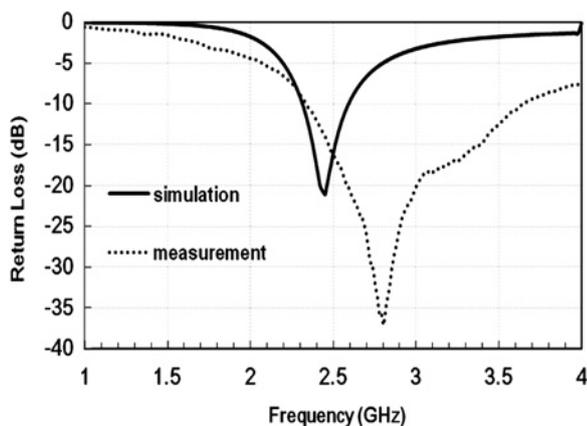
**Fig. 6** Return loss of the SAW-based RFID tag
