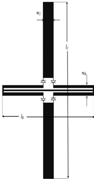
**Fig. 8** Layout of the crossed-dipole frequency-doubling tag operating between  $f_0 = 3.5$  GHz (interrogating frequency) and  $2f_0 = 7$  GHz (tag response)
