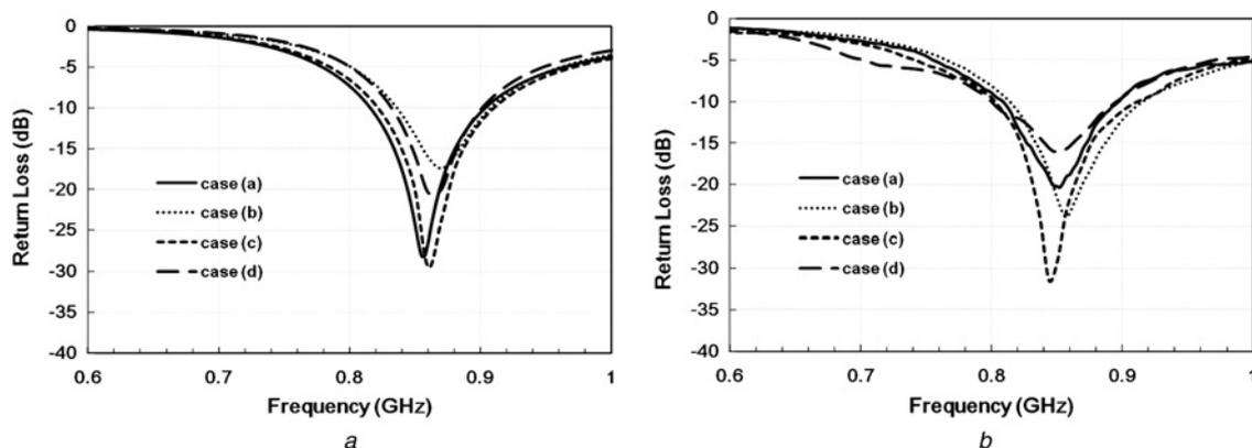
**Fig. 2** Return loss comparison of the four inkjet-printed antenna designs at European RFID band
