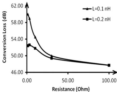
**Fig. 16** Conversion loss trend for different resistance and inductance values ( $P_{in} = -30$  dBm)
