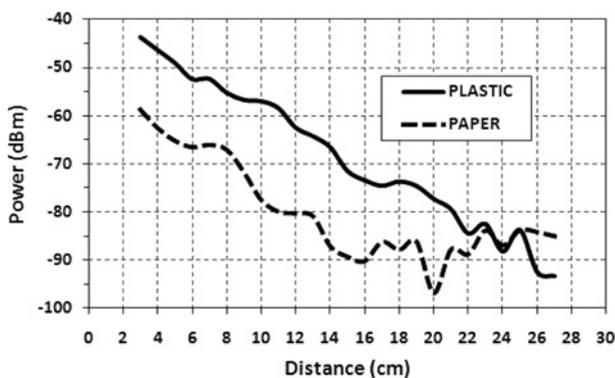
Fig. 12 Received power against the distance for the crossed-dipole frequency-doubling tag
