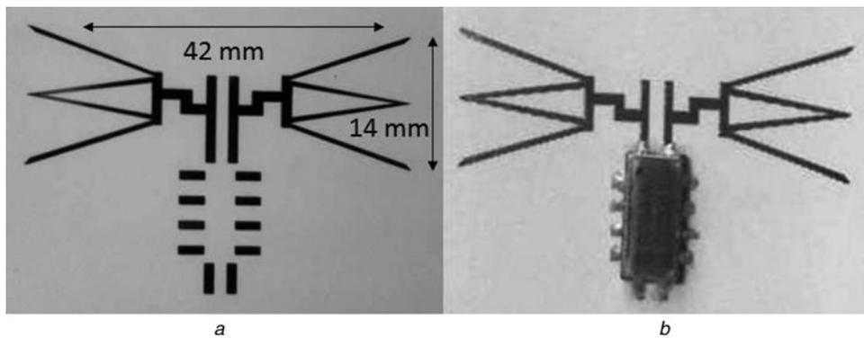
**Fig. 5** Photograph of the inkjet printed antenna and circuit and photograph of the same printed sample with the mounted SAW based RFID
