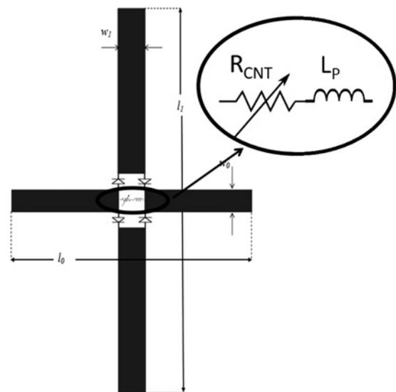
Fig. 14 RF enabled sensor node concept
