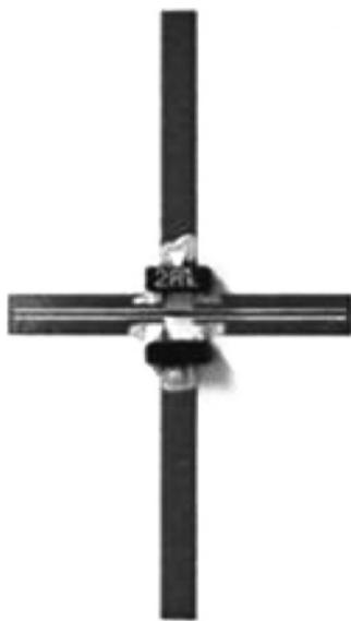
**Fig. 9** Photograph of the crossed-dipole frequency-doubling tag based on paper substrate
