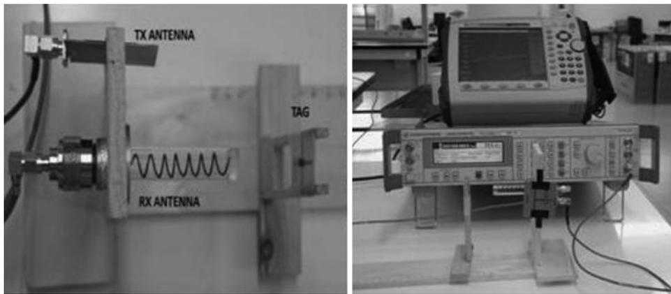
Fig. 10 Measurement set-up for the frequency-doubling tag
