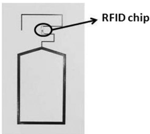
**Fig. 4** Photograph of the proposed inkjet-printed RFID tag on paper-based substrate with ink-usage after the ink optimisation
