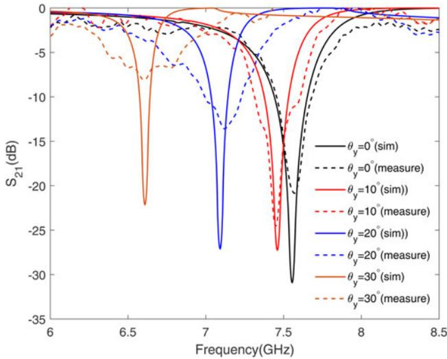
Fig. 10. Horizontal polarization ( $x$ -axis) with different  $y$ -axis rotating angles simulation and measurement results.
