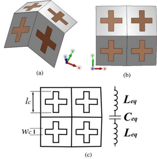
**Fig. 3.** Design of cross-dipole eggbox FSS element: (a) perspective view; (b) top view; and (c) equivalent circuit.
