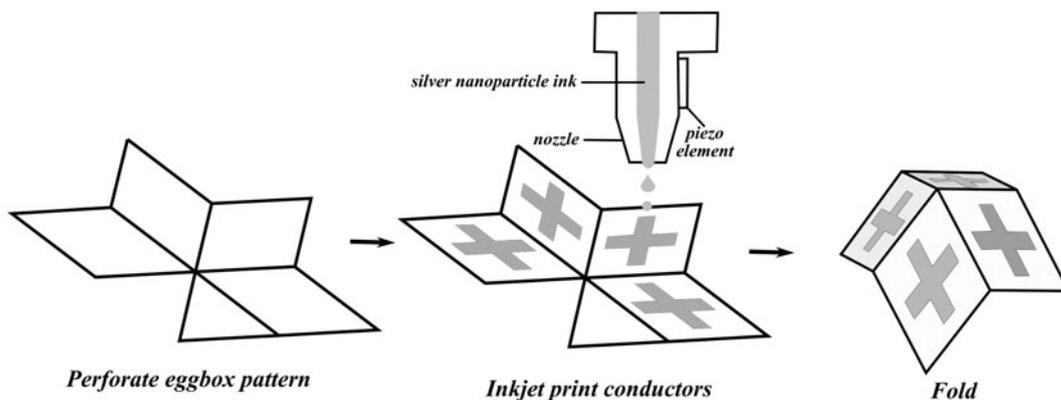
Fig. 5. Three-step fabrication process for eggbox FSS: perforate eggbox pattern; inkjet print conductive traces; and fold to 3D eggbox structure.
