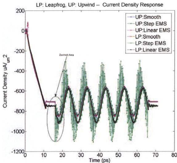
Fig. 5. Current density response to the reference excitation, a piecewise linear approximation and a stepwise linear approximation. The piecewise linear approximation and the reference excitation are similar; however the stepwise approximation shows significant overestimation in the change induced by the excitation.
