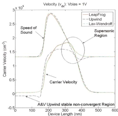
Fig. 3. Steady-state Velocity profile of *n-i-n* diode models showing the non-physical convergent results for the *Upwind* method when the ramp excitation rate is too steep.
