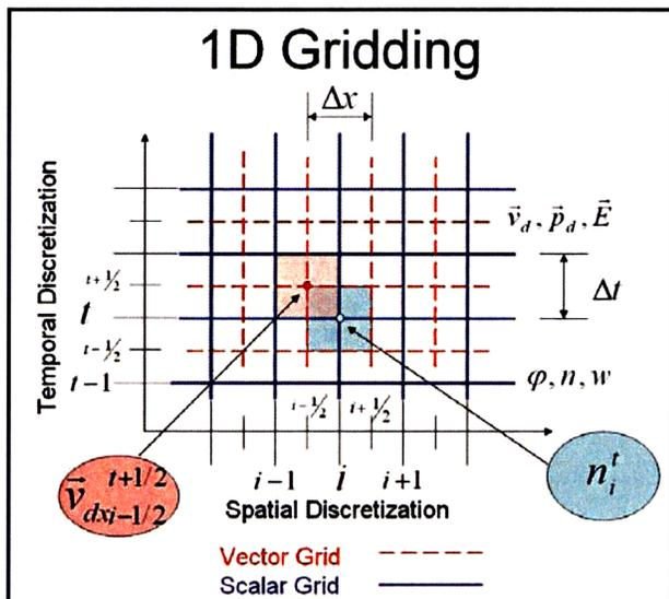
Fig. 1. Staggered Gridding technique showing vector and scalar offsets in time and space.
