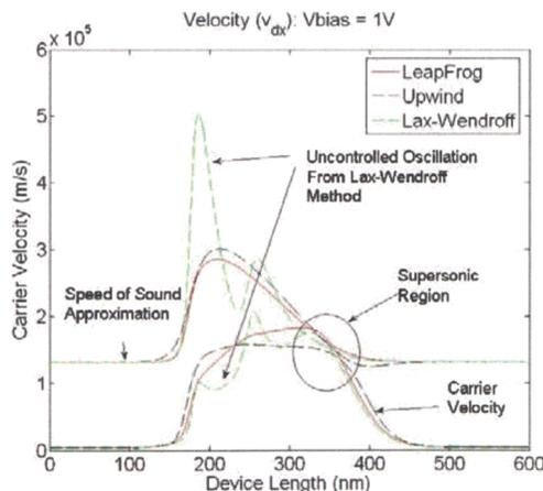
Fig. 4. Steady-state Velocity profile of *n-i-n* diode for a much slower ramp excitation and much longer execution time. The *Lax-Wendroff* method tends to oscillate when sufficient execution time has elapsed.
