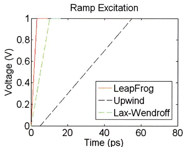
Fig. 2. Maximum stable ramp excitations showing the maximum ramp rates the produced reasonably stable or convergent solutions.
